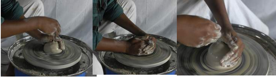
Centring - force the clay to the centre of the wheel by applying pressure with the hands
