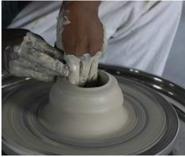
Hollow and Levelling
