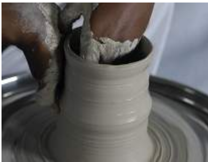
Lifting up the wall
