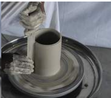
Levelling the wall with the ruler
