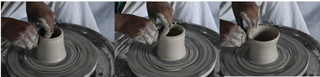
Lifting the wall of the cylinder
