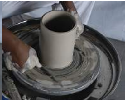
Cut the completed Cylinder using wire
