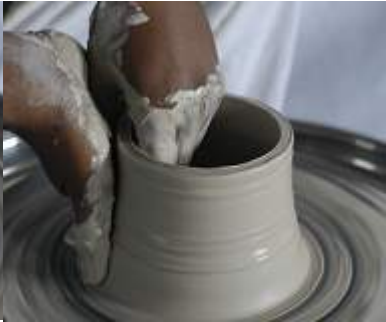
Lifting up the wall
